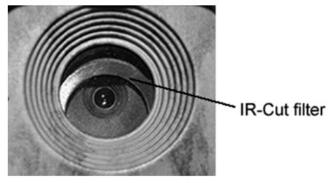
A: The camera is not broken. It's an IR-cut filter. When the camera is powered on, the IR-cut will be reset and cover the lens. Only when the camera is powered off, the IR-cut will be at a random place.
